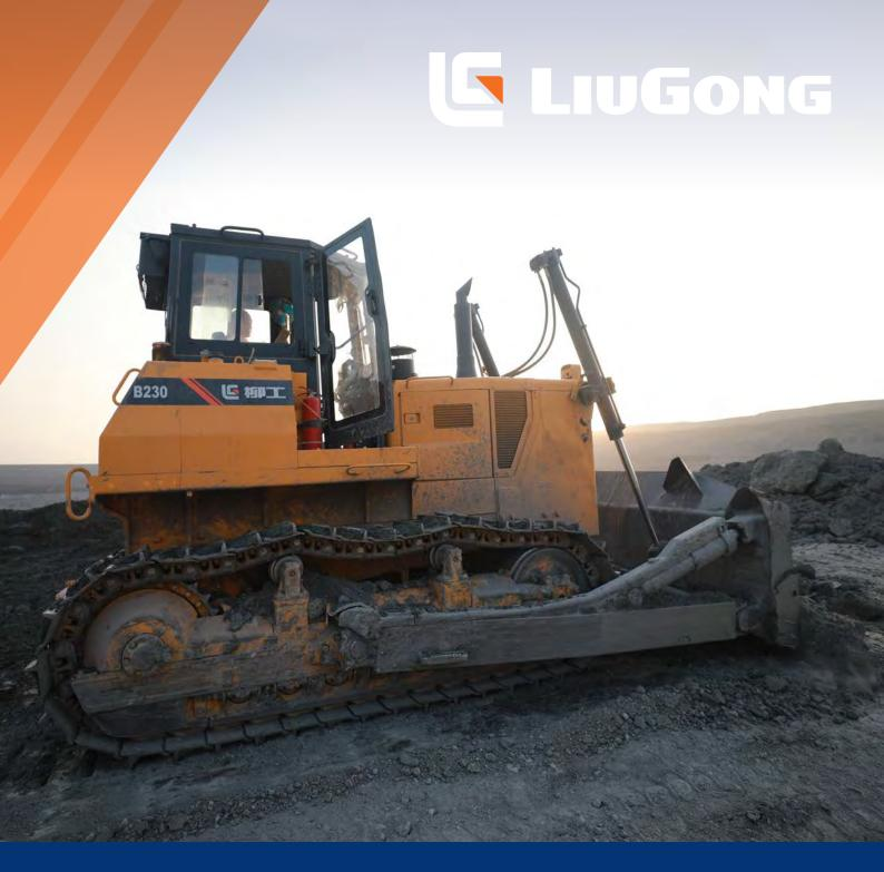
Engine ChongQing Cummins Gross Power 179 kW (240 hp / 243 ps) @ 2,000 rpm Net Power 169 kW (227 hp / 230 ps) @ 2,000 rpm Maximum Torque 1,050 N  $\cdot$  m Blade Capacity 7.8 m³ Operating Weight 24,540 kg
